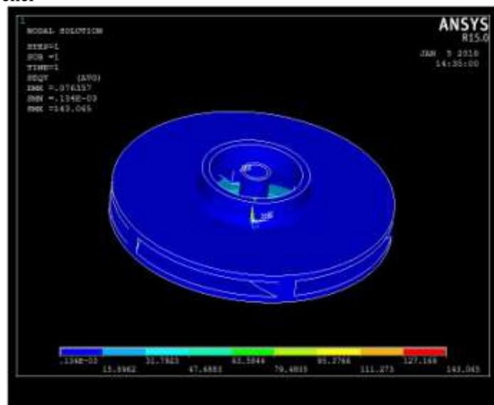
**Fig.- 9** Stress distribution for steel impeller
