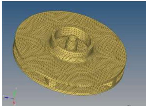
Fig:5 tetra-hedral meshing of pump impeller
