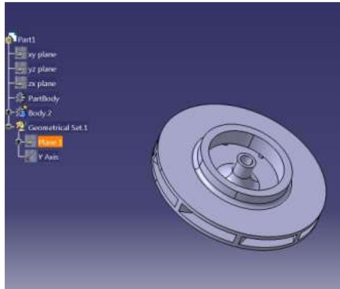
Fig 4. 3D CAD model of impeller
