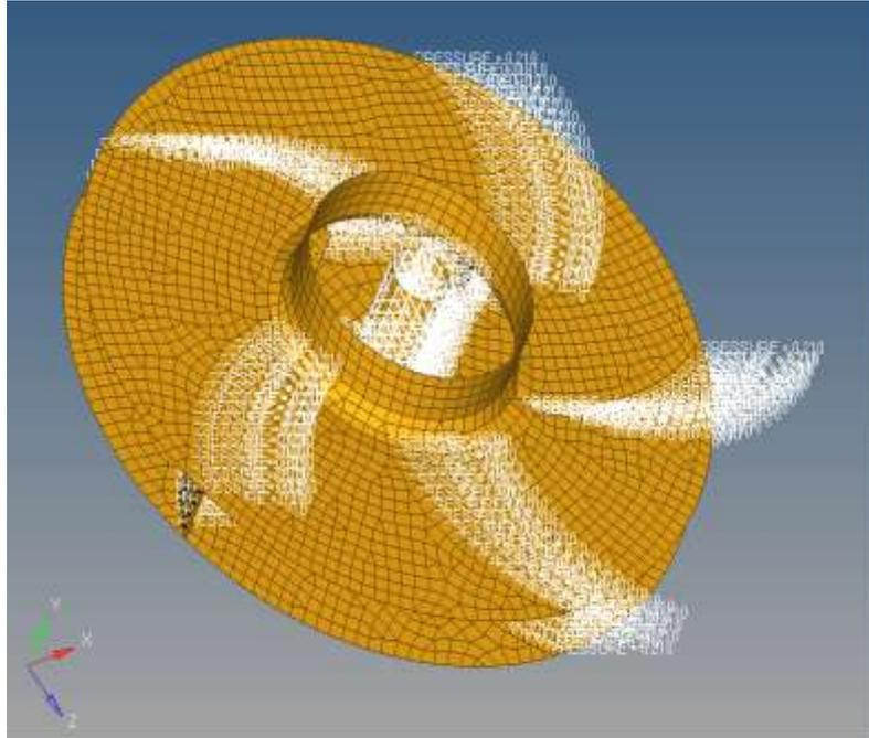
**Fig.-10** Loading and boundary conditions when pressure applied on all blades
