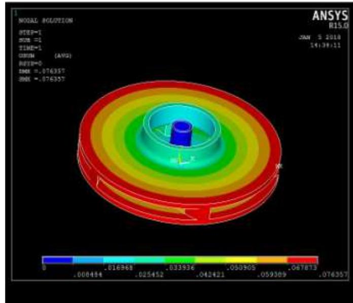
**Fig.8** Deformation for steel impeller
