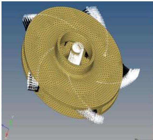
**Fig.-7** Loading and boundary conditions
