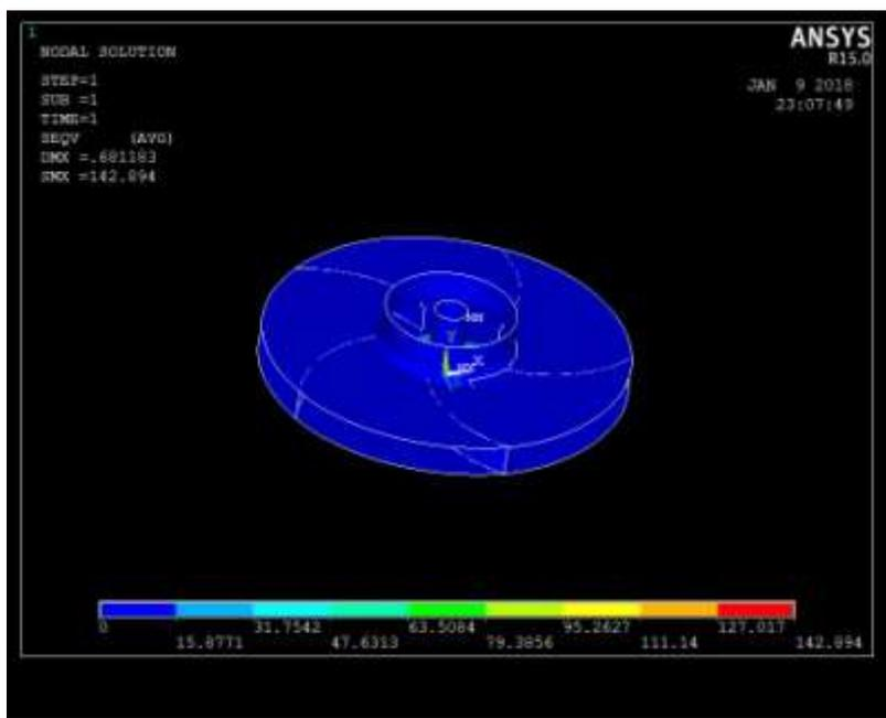
Fig.12 stress plot for composite impeller
