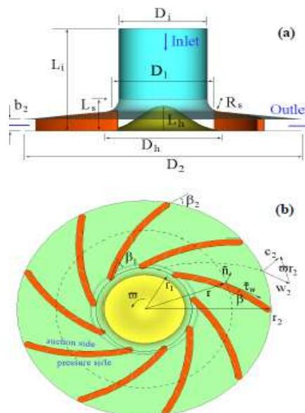
Fig:3 Details of impeller geometry
