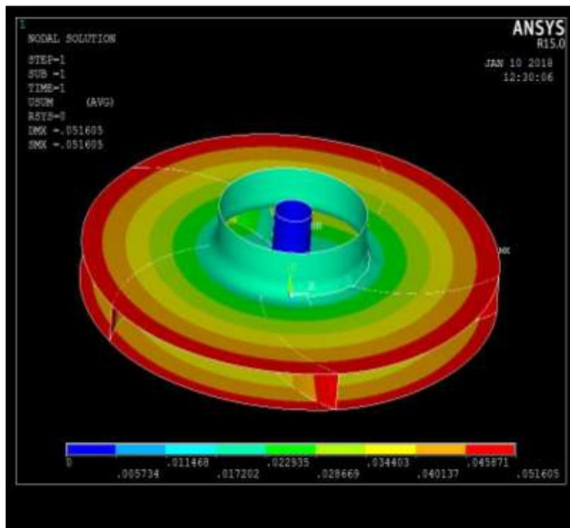
**Fig 11** Deformation of composite impeller
